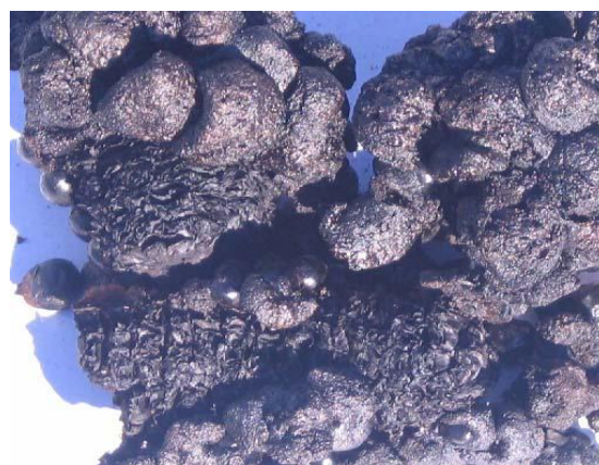
Fig. 2. The texture after thermic treatment of the dried vegetal remains from maize
