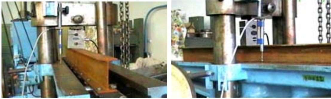
a b Fig. 8.32 Experimentally assembly 1.c Case a-steel beam transverse applied, b-assembly depth
