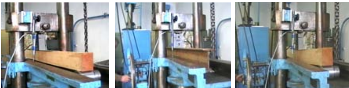
a b c Fig. 8.33 Experimental Assembly for the reference beams (Case 1.b and 1.c) a- wood beam (reference for 1.b Case), b-steel beam (reference for 1.c Case), c-wood beam (reference for 1.b Case), applied and distorted. c-
