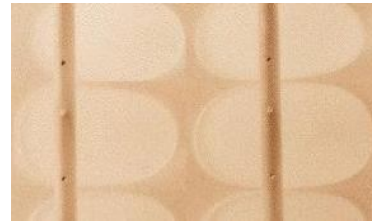
The deposition of dust on the deposition electrode next to the emission electrode Isodyn B5 (a) and Isodyn B5M (b)
