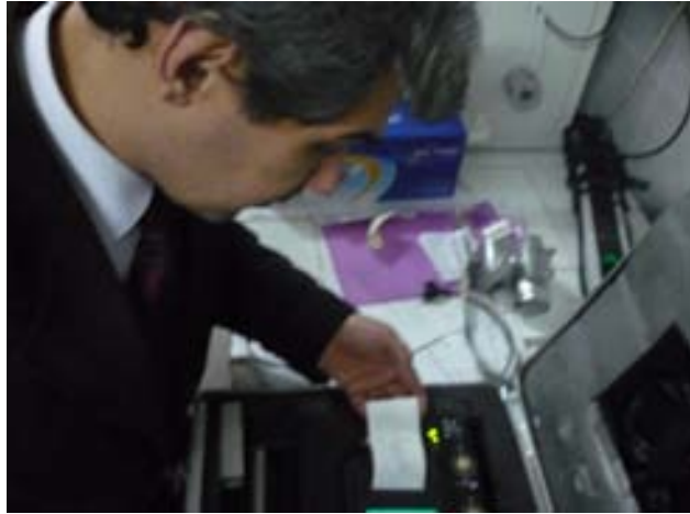
Figure 2 - Assessment of concentrations of CO, CO 2 and NO x from measurements made with TESTO 350 M / XL
